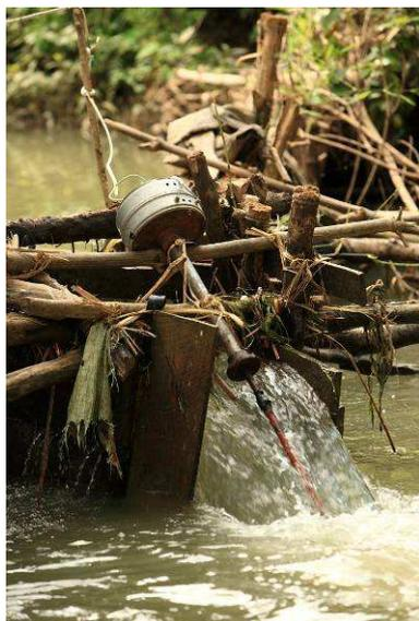
**Fig. 2** Pico-hydropower turbine
